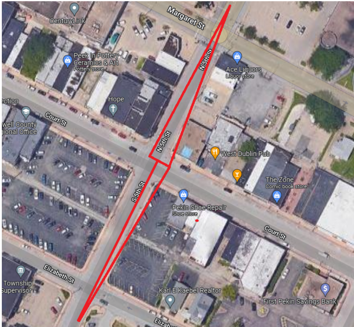
Figure 16– Sight distance Triangles for westbound Court Street traffic
