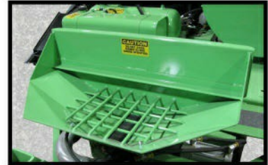
The hopper receives aggregate from the dump truck.
