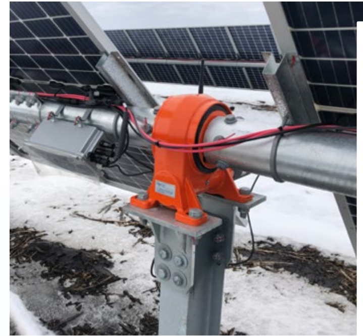
Example of single-axis tracker system in summer.
