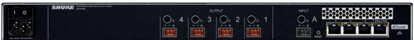
MXWANI4 4-Channel Audio Network Interface: Rear Panel
